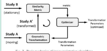
Fig. 2. Basic mechanics of image registration algorithms.
